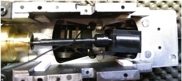
2. We fitted the Zimo LS40x22x09, as this was just the right width and height to fit in without causing a problem with clearance. The Rail Exclusives one is just a little bit too high at 10mm to give adequate clearance in all models
