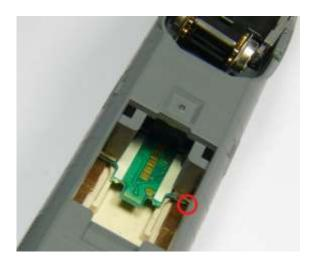
The ZIMO Decoder MX605SL is inserted into the shaft with tweezers. It comes to rest between the contact plates. Make sure that the decoder is pushed to the front oft he shaft.
