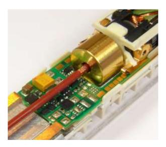
As in the Kato instructions, the cardan shaft is pulled out of the cardan shell of the bogie. The same is done afterwards on the motor side. The ZIMO Decoder MX605N is inserted with the yellow tantalum capacitor "up" (to the viewer). The cardan shaft and the car body is assembled in reverse order.
