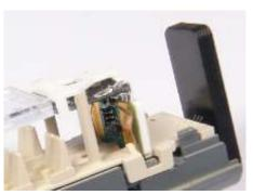
The ZIMO Decoder MX605FL is placed on the decoder holder. Both are then pushed between the contact plates and the plastic holder until the decoder holder engages in the car interior.
